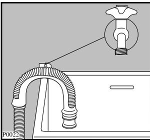
**In a sink drain pipe branch.** This branch must be above the trap so that the bend is at least 60 cm above the ground.
